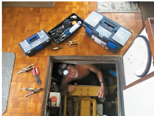
The day after the big zap, Bill was in the engine room hunting down lightning damage. The fuse on the old transient voltage-spike protector had disintegrated
