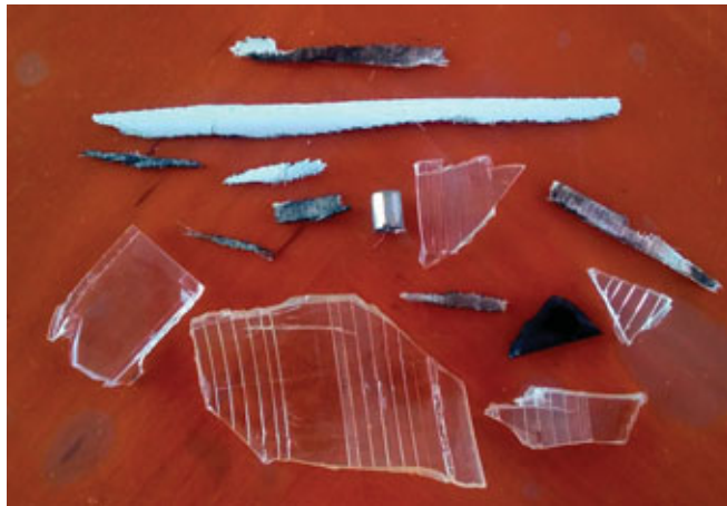
Clockwise from left: On Ultra's buddyboat, the lightning left shattered shards of nav lights and the burned plastic VHF antenna
